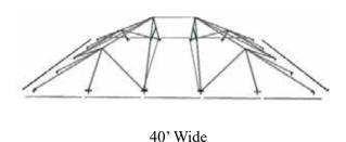
3. Start at one corner of the frame and insert and pin the Corner Fitting to the Spreader. Continue in one direction around the frame inserting and pinning each fitting to the Spreaders.
