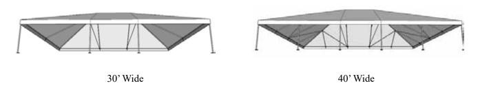
6. Lift the other side of the tent and attach the legs (with base plates). While this unit will stand on its own, it is NOT intended that the base plates be used as an anchoring method. The stakes should be driven approximately 5 feet away from the bottom of the leg. It is imperative the tent be secured with ropes and stakes or any other appropriate anchoring method. It is recommended that you do not bolt the base plates to any surface. Store the cover only when clean and dry.
