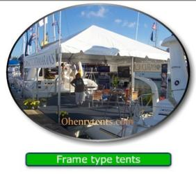
The frame type tent is ideal for use indoors where staking is not possible, or in applications where a center pole is undesirable. or the tent needs to be installed against a building. Frame tents should be staked out just like a pole tent when used outdoors.
