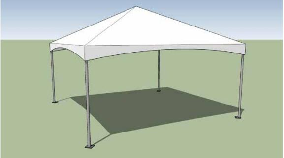
8. At each leg, now drive a tent stake into the ground about 5' from the edge of the tent. Attach the Guy Ropes provided with your tents and tighten securely to the tent stake. provided. In the event of high winds, the cover should be removed from the frame to prevent damage to your tent. Your tent should be vacated during inclement weather.
